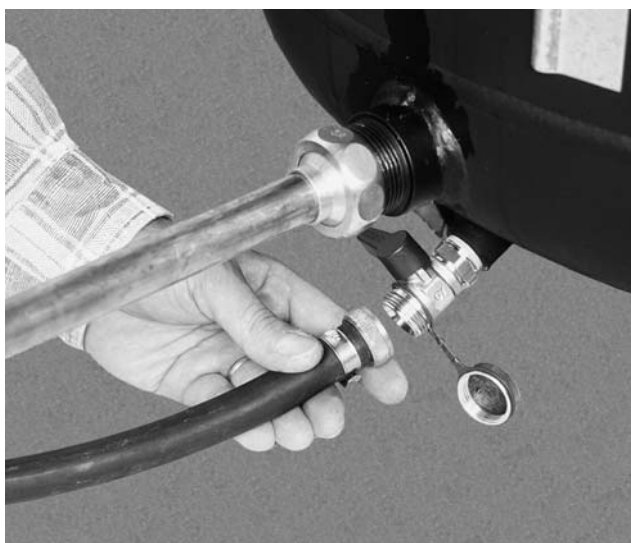
Figure 16 For the initial startup, connect filling/emptying cock with hose at bottom of storage tank and allow water to flow into the cylinder. Then open filling/emptying cock at the top where the cover is to allow air to escape.
